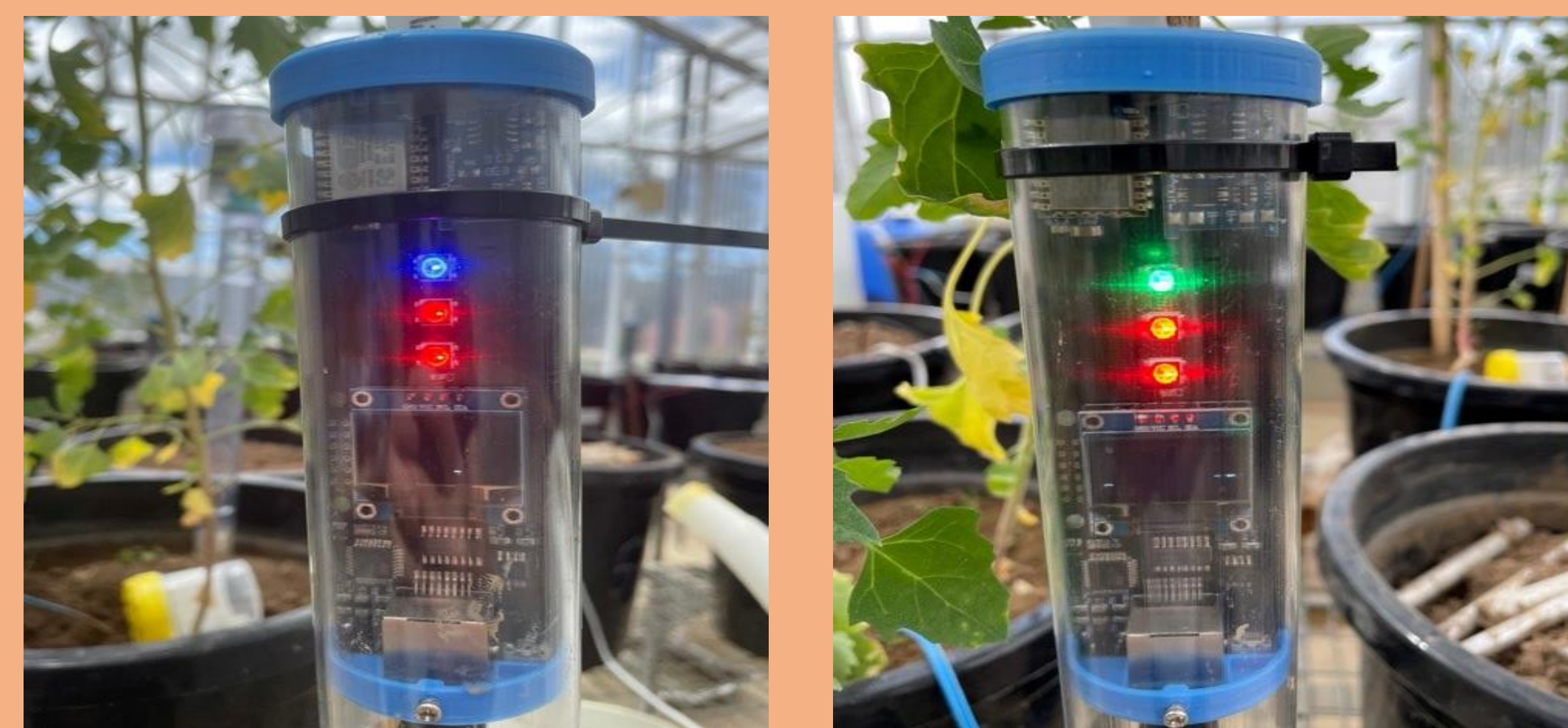
Fig 3: Chameleon soil moisture sensors
